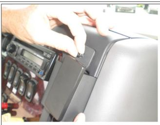
2. Align the upper hole in the ProClip over the screw hole in the dash. Push the panel frame back into place and screw the screw just a few threads into the screw hole.
