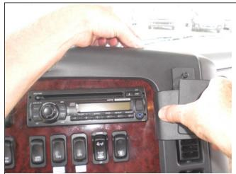
3. Using your left hand again, pull the panel frame slightly towards you. Then push forward on the left side of the ProClip so the angled edge hooks around the panel frame edge. Push the panel frame back into place and secure the frame and the ProClip by tightening the screw.
